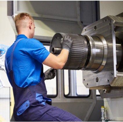
Radial run-out measurement on an HSTR main spindle
