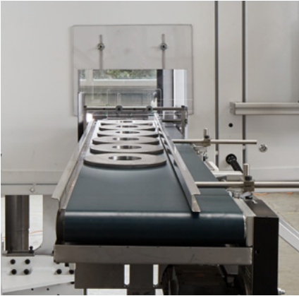
Feed belt / buffer storage unit on a VSTR
