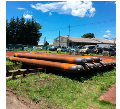
Typical jumbo cylinders produced on an RVM 600
