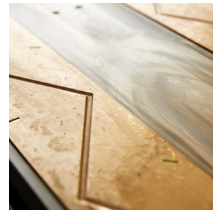
A special feature of our industry: Hand-formed bronze slideways
